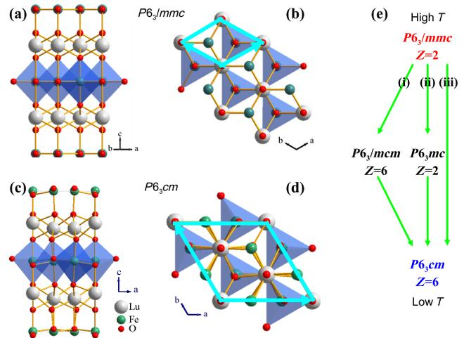
FIG. 2 (color online). The schematic representation of  $P6_3/mmc$  and  $P6_3cm$  structures and the possible transition routes. (a) and (b) are the  $P6_3/mmc$  structure viewed from the [120] and [001] directions, respectively. (c) and (d) are the  $P6_3cm$  structure viewed from the [100] and [001] directions, respectively. The bold lines in (b) and (d) indicate the unit cells in the  $a$ - $b$  plane. (e) Possible routes from  $P6_3/mmc$  to  $P6_3cm$  structures.
