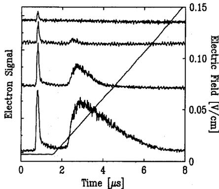
Fig. 1. Electron signals for four different dye-laser pulse energies, which produced charged-particle densities from  $10^5$ – $10^7 \text{ cm}^{-3}$ . The laser fires at  $t = 0$ , and the initial kinetic energy of the photoelectrons is  $0.4 \text{ cm}^{-1}$ . Also shown is the field ramp applied 1.6  $\mu$ s after the laser pulse. The signal at 1  $\mu$ s is the prompt photoelectron signal, and the signal after 2  $\mu$ s is from the plasma (from Ref. 3).
