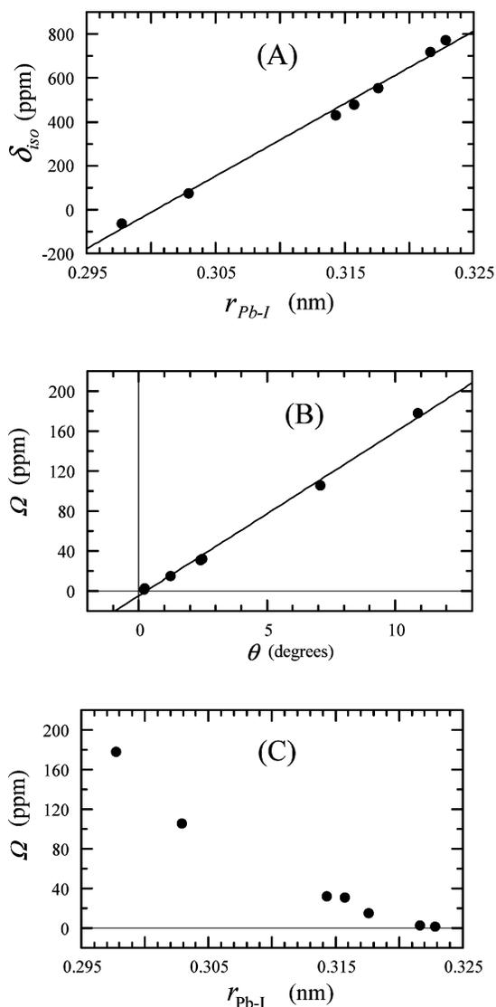
**Figure 9.** Calculated NMR parameters of a  $\text{PbI}_6^{4-}$  cluster using ZORA-DFT techniques. (A)  $\delta_{\text{iso}}$  versus  $r_{\text{Pb-I}}$ , (B)  $\Omega$  versus  $\theta$ , and (C)  $\Omega$  versus  $r_{\text{Pb-I}}$ .
