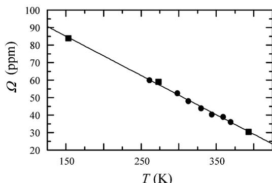
**Figure 3.** The temperature  $T$  dependence of the span  $\Omega$  for  $\text{Pb}(\text{NO}_3)_2$ : ●, 62.6 MHz (this work); ■, ref 29. The solid line is the best-fit linear relation as given in eq 6 with the parameters given in Table 1.
