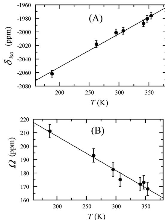
**Figure 4.** The temperature  $T$  dependence of (A) the isotropic chemical shift  $\delta_{\text{iso}}$  and (B) the span  $\Omega$  of  $\text{PbMoO}_4$  determined at 62.6 MHz. These parameters are obtained from fitting the experimentally obtained spectra as indicated in Figure 1. The solid lines are the best-fit linear relations as given by eqs 5 and 6 in the text.
