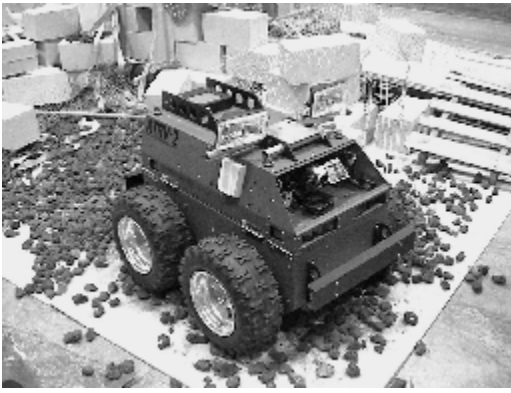
Figure 1: NIST's USAR arena. This picture shows one of the "hard" areas. Note the debris and ramps that make it difficult for autonomous robots.
