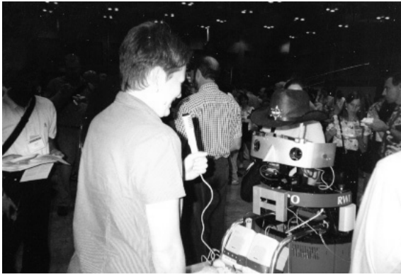
Figure 3: Elektro dishes out cookies and conversation while attempting to re-recognize conference attendees using our multi-modal color histogram technique.
