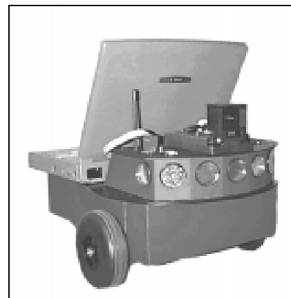
Figure 1: The mobile robot with laptop controller and CCD camera.
