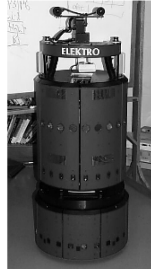
Figure 6: Elektro the robot. Elektro is a Real World Interface, Inc. B21 robot. It has sonar, laser, infrared, and tactile sensors, as well as a high-performance stereo vision system. Here it is shown without its candy dispenser, which sits directly behind the cameras.
